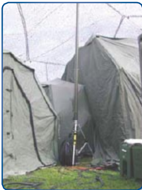
As an option, the composite push-up masts can also be used as CAMO POLE tent pole supports.
